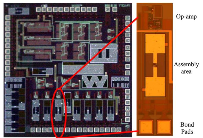
Fig. 1 Optical photograph of the CMOS chip.
