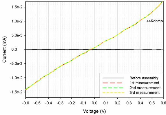
Fig. 4 Two terminal I-V measurements from assembled SWNTs.
